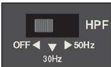
A filter having a passband extending from some finite cutoff frequency (not zero) up to infinite frequency. Also known as a low-cut filter. HPF rolls off signals below 30Hz or 50Hz, removing the frequencies below the selected roll off. Reproduction of the signal’s bass portion is thus optimized, since ultra-low, distracting frequencies are eliminated, and more power is available for the reproduction of the wanted segment of the signal.
